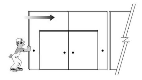
Step 1: Engage the mechanism located on face of the panel closest to you by placing operating key in face opening and turning one half revolution.
