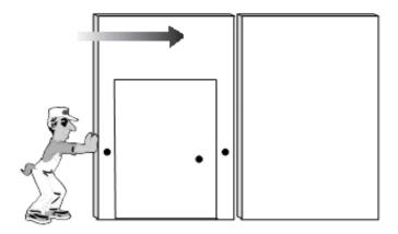
Step 1: Engage the mechanism located on face of the panel closest to you by placing operating key in face opening and turning one half revolution.
