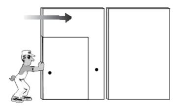
Step 1: Engage the mechanism located on face of the panel by placing operating key in face opening and turning one half revolution.
